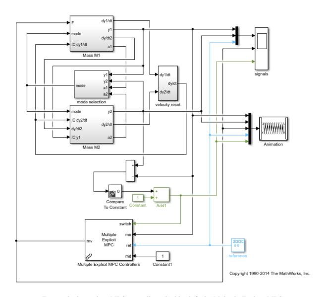
To specify the explicit MPC controllers, double-click the Multiple Explicit MPC Controllers block. In the Block Parameters dialog box, specify the controllers as a cell
