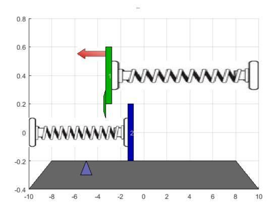
Both masses move freely until they collide. The collision is completely inelastic, and the masses stick together until a change in the applied force separates them. Therefore, there are two operating conditions for the system with significantly different dynamics.
