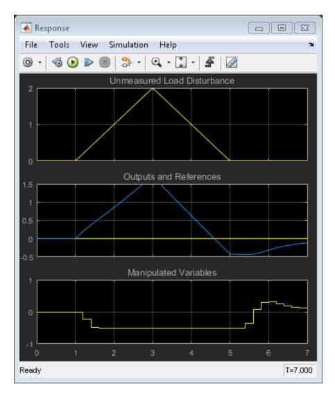
The plant input and output signals are identical to those obtained using the built-in Model Predictive Control Toolbox solver, but the qp.status shows that quadprog does not take the same number of iterations to find a solution. However, it does detect the same infeasibility time period.
