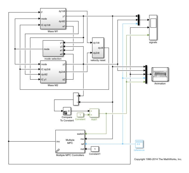
In the model, the Mass M1 subsystem simulates the motion of mass M1, both when moving freely and when connected to M2. The Mass M2 subsystem simluates the motion of mass M2 when it is moving freely. The mode selection and velocity reset subsystems coordinate the collision and separation of the masses.
