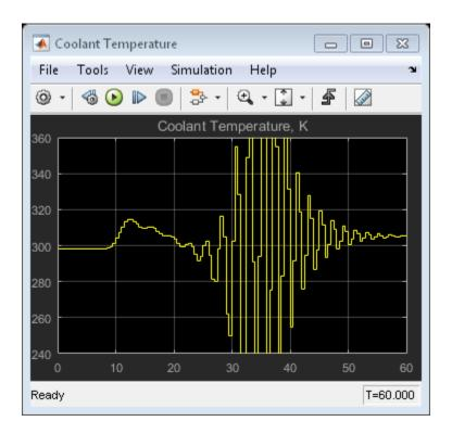
The closed-loop response is unacceptable. Performance along the full transition can be improved if other MPC controllers are designed at different operating conditions along the transition path. In the next two section, two additional MPC controllers are design at intermediate and final transition stages respectively.
