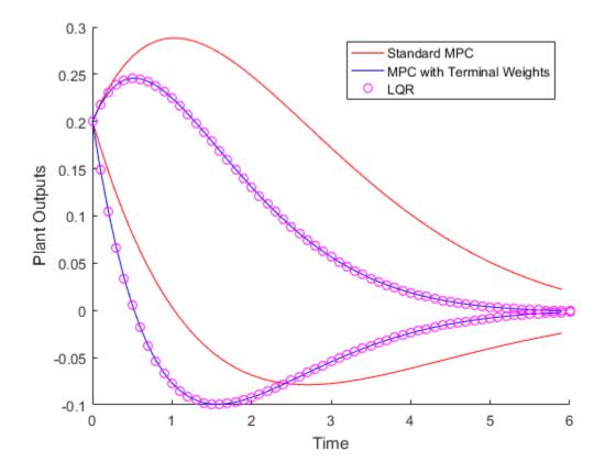
The MPC controller with terminal weights has a faster settling time compared to the standard MPC controller. The LQR controller and the MPC controller with terminal weights perform identically.
