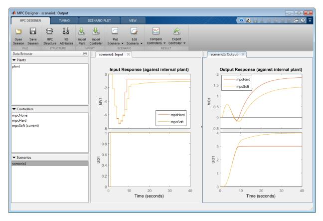
You can toggle the display of any controller in the **Data Browser** except for controller currently being tuned. Under **Compare Controllers**, the controllers with displayed responses are indicated with check marks.
