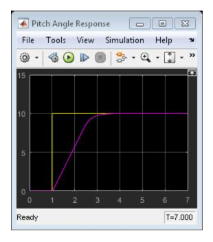
The closed-loop response is identical to the traditional MPC controller designed in the "mpcaircraft" example.
