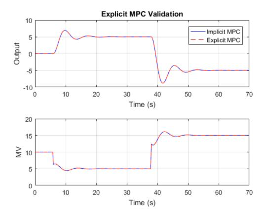
The closed-loop responses and manipulated variable sequences of the implicit and explicit controllers match. Similarly, you can validate the performance of expMPC2 against that of MPC2.
