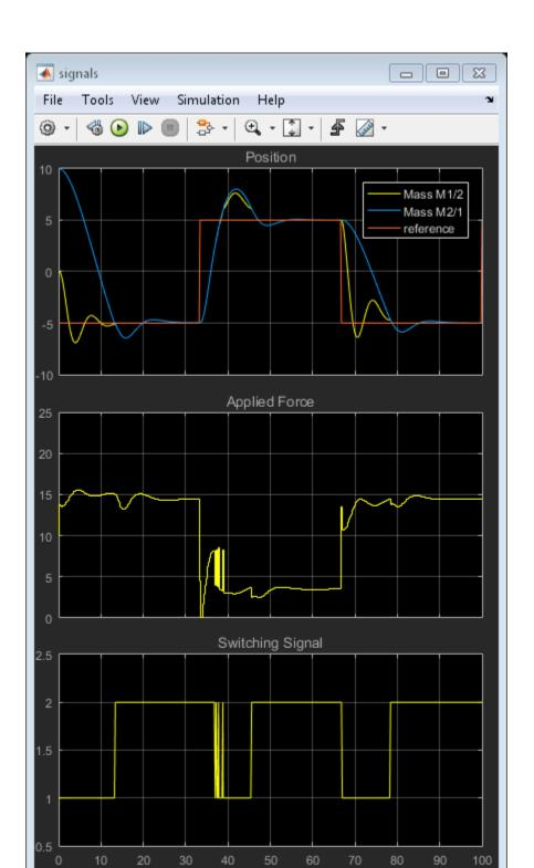
Initially, MPC1 moves mass M1 to the reference setpoint. At about 13 seconds, M2 collides with M1. The switching signal changes from 1 to 2, which switches control to MPC2.
