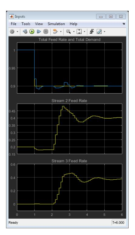
The MPC controller controls the blending process. The block labeled Blending incorporates the previously described model equations and includes an unmeasured step disturbance in the constituent 1 feed composition.
