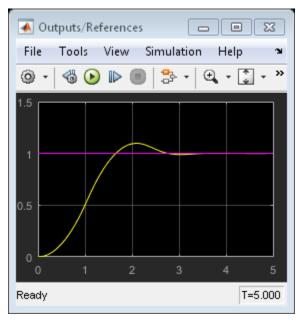
Simulate with Explicit MPC controller in Simulink. Controller "mpcobjExplicitSimplified" is specified in the block dialog.
