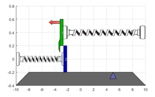
When the masses are not connected, MPC2 applies excessive force since it expects a larger mass. This aggressive control action produces oscillatory behavior. Once the masses connect, the control performance improves, since this is the condition for which the controller is designed.
